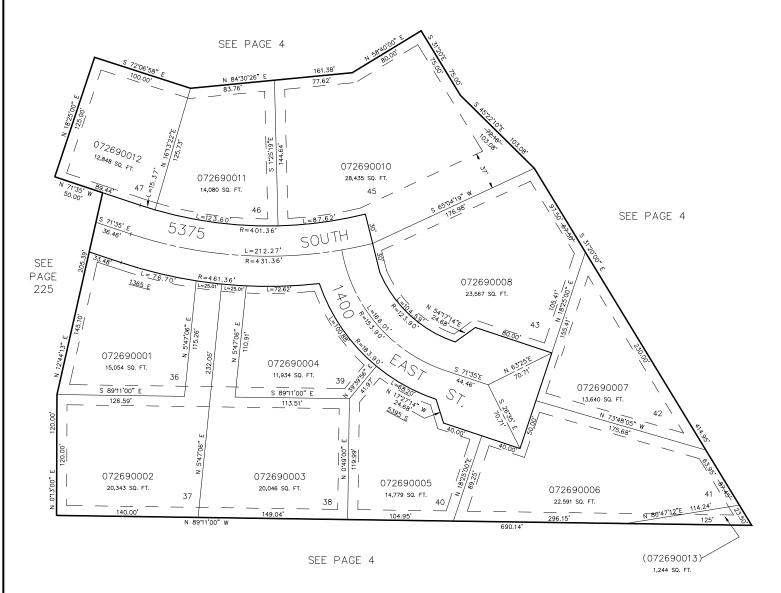
10' UTILITY EASEMENTS EACH SIDE OF PROPERTY LINE AS INDICATED BY DASHED LINES. ALL ESMTS TO BE USED FOR IRRIG. WATERLINES, DRAINAGE, SANITARY & STORM SEWERS, POWERLINES, TELEPHONE LINES & OTHER PUBLIC UTILITIES. FRONT PROPERTY LINE UTILITY EASEMENTS ARE 7' MIDE. OTHERS AS SHOWN.
